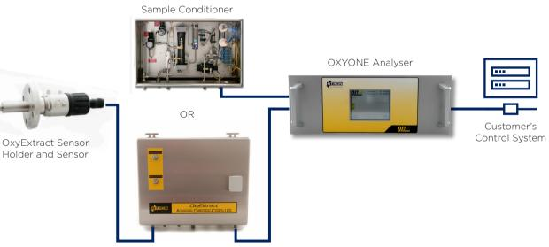
Automatic Calibration Control Unit (ACCU) with OxyExtract
